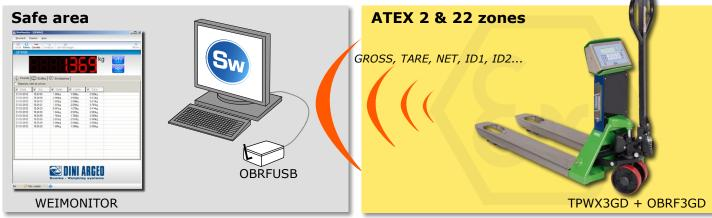
Weighing platform in Ex 2 or 22 areas connected to an ATEX weight indicator with transmission of the weight through OBRF3GD radio modules to repeaters at a distance, inside the same ATEX area.
